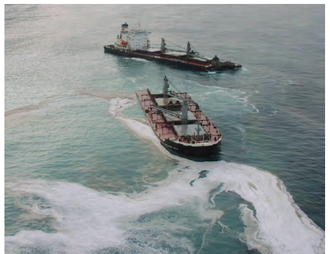
▲ Figure 13: Heavy fuel oil spilled as a result of the catastrophic failure of a bulk carrier. The cargo has mixed with the oil making realistic estimations of the volume of spilled oil difficult to determine.
