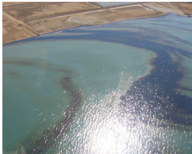
▲ Figure 21: Light reflection off the sea can sometimes be a problem when taking aerial photographs; UV and polarising filters may help to sharpen the visual definition of oil.
