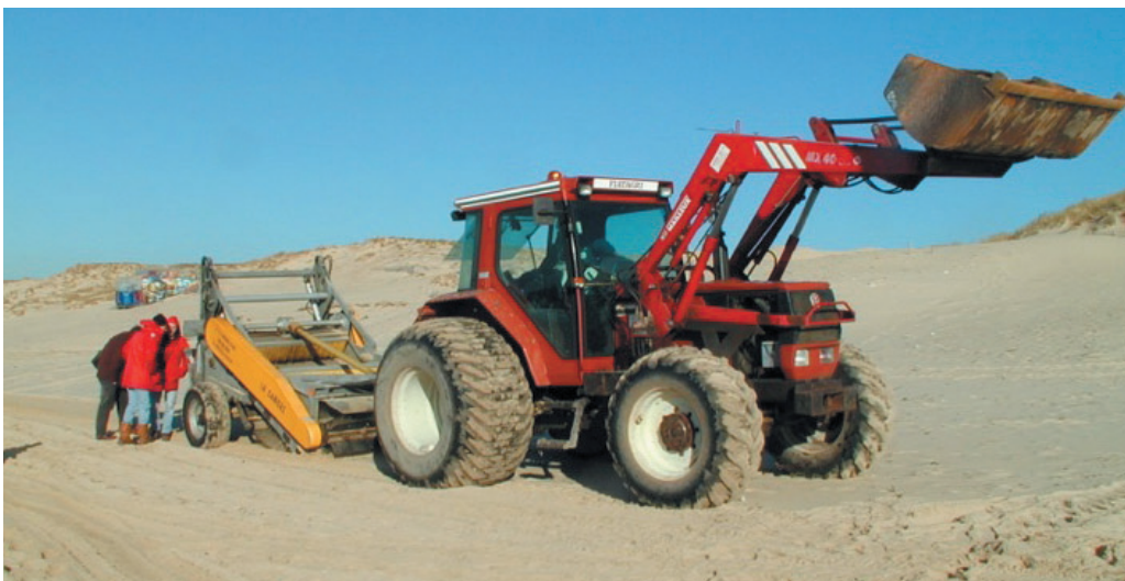
A tractor-towed beach-cleaning machine
