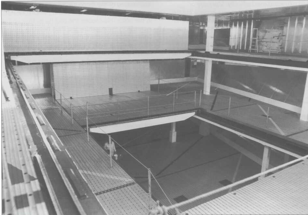
View into a refrigerated cargo hold
