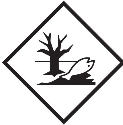
FIGURE 7.1.B Environmentally Hazardous Substance Mark (7.1.6.3)
