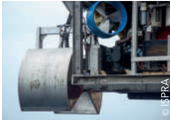
Grab sampler mounted on a Class II ROV
