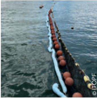
Custom-made boom made from nets and sorbents for a Palm Stearin spill
