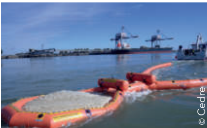
Dynamic containment with a Current Buster
