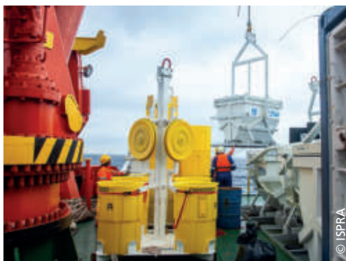
Specific racks where recovered drums were placed on sea bottom by a work class ROV
