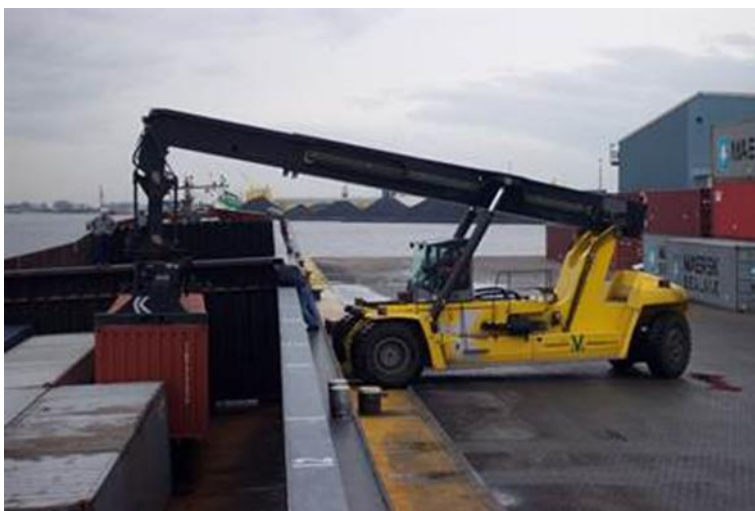
Figure 5: Loading and unloading of an inland water container ship with a reach stacker
