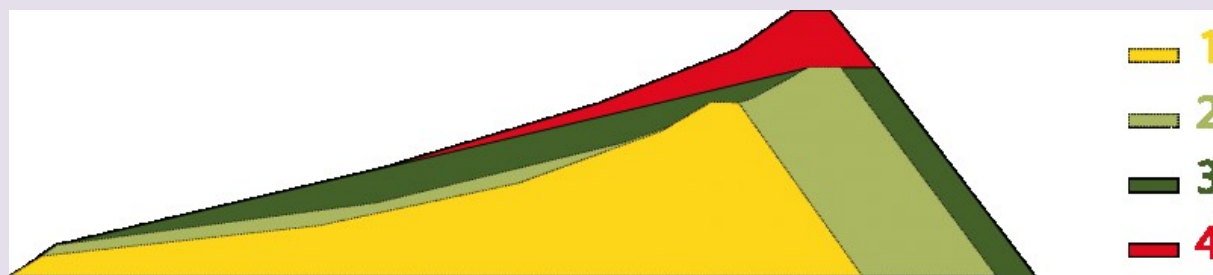
1) Existing Dyke, 2) Dyke reinforcement with a climate surcharge of 0.5 m, 3) Adapted dyke profile for construction reserve, 4) Construction reserve for additional heightening in case of a more severe sea level rise
