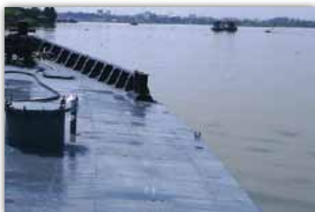
Figure 95: Absence of Fence and Spill Belt on Low-Standard Tanker Barge
