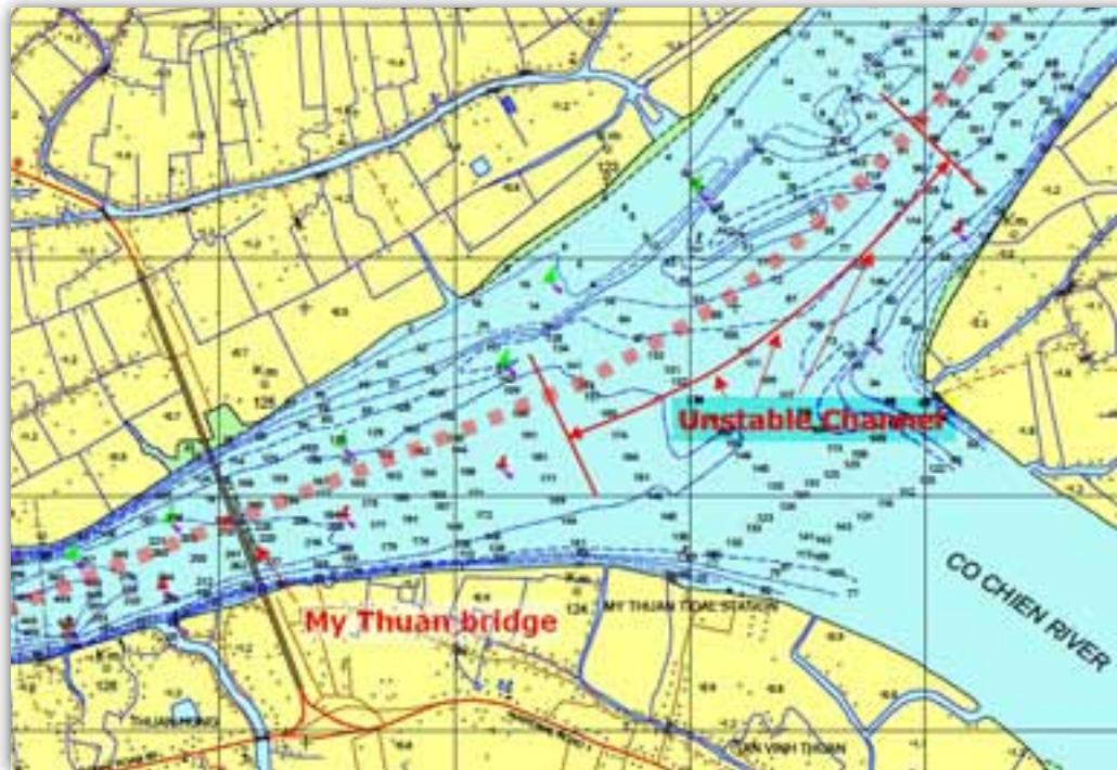
Figure 150: Unstable Channel Near Entrance of Co Chien River
