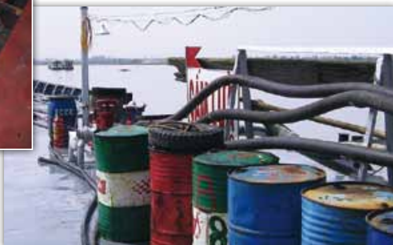
Figure 94: Deck Arrangement on Low-Standard Tanker Barge
