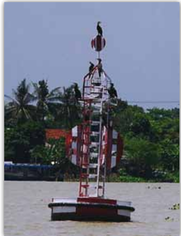
Solar panels from buoys (left) are supposed to recharge batteries during the day. But they are often stained by bird droppings and no longer working. The “safe water” buoy (right) seems to be a favourite gathering place for birds.
