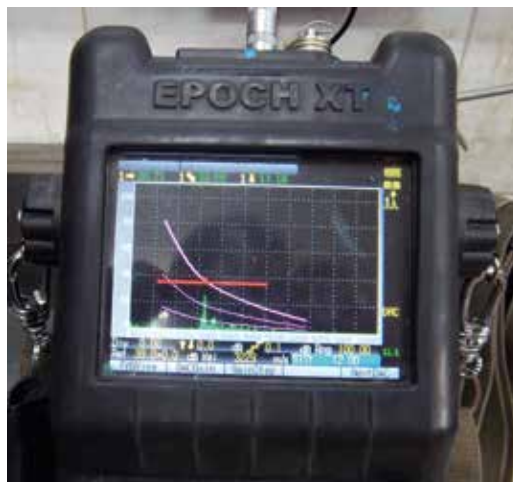
NDT testing using ultrasonic flaw detector
