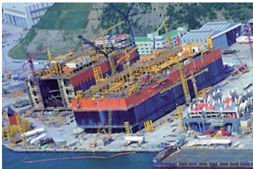
Figure 9. FPSO unit built on ground.
