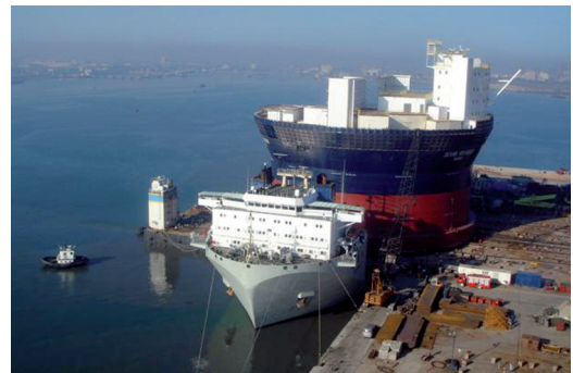
Figure 10. SSP built on ground and transferred to special barge.
